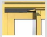
To ensure the opening door panel stays on the track when opened we fit a tapered buffer stop into head frame.
